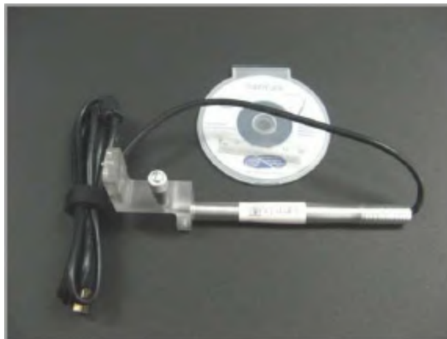
Figure 9 Micrometer/camera Assembly
